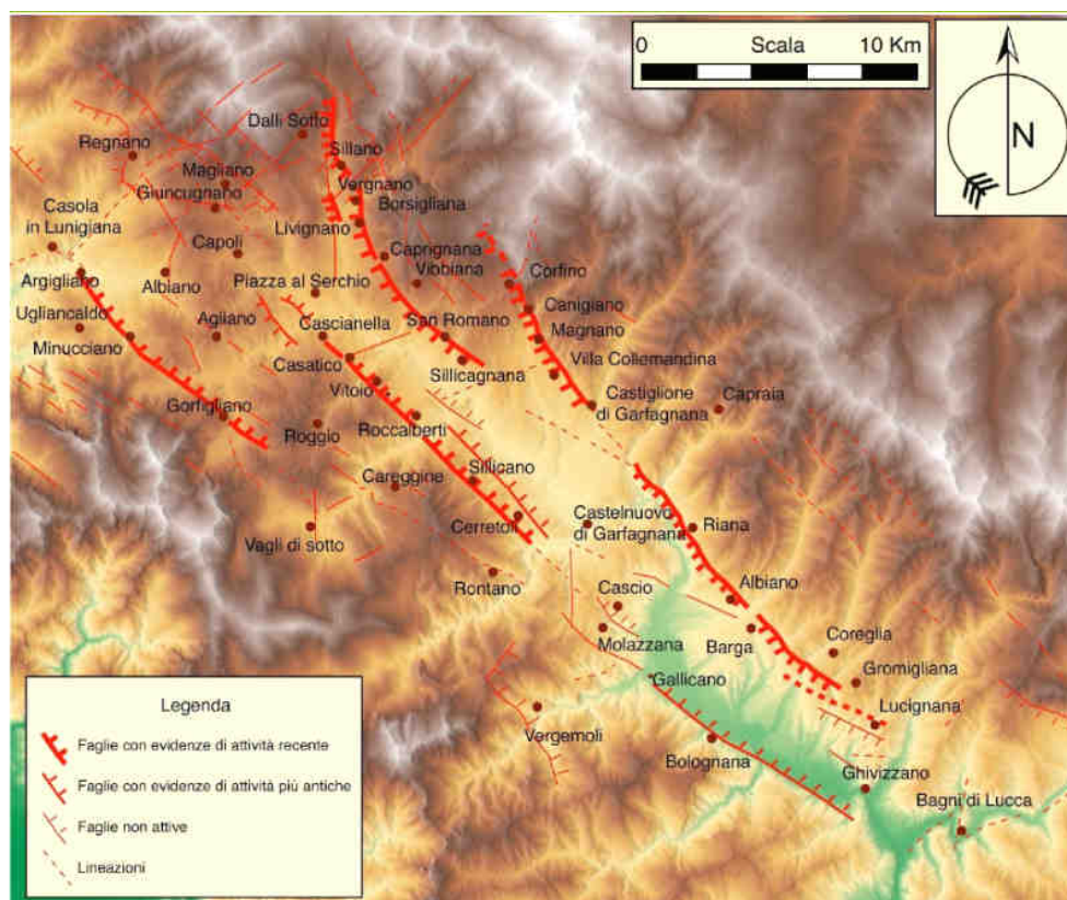
Principal faults of the mid-upper Serchio Valley from published literature combined with original fieldwork, analysis of aerial photos and analysis of DEMs (from Vannucci [1999]).
